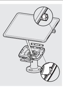
Remove the Fixing Covers. Feed the Flat Cable into the assembly & locate the Tablet in the chosen
