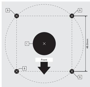
Mark 'B' positions for "Fixing from below" (Ø5.0mm drillbit). Mark 'C' for routing the cable hole. (Ø20.0mm Holesaw).
