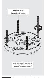
Screw in the 4x Socket **B2** Set Screws. Ensure full thread engagment.
