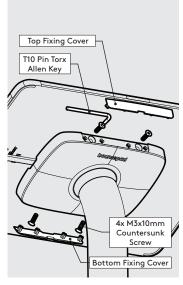
Secure the Tablet to the 10 Shell & attach the Fixing Covers as shown.
