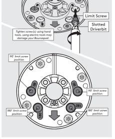
Configure the rotation range - both arrows must point in the same direction. Default configuration is 270°. Insert 2x limit screws.
