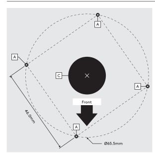
Mark 'A' positions for "Fixing from above" (Ø2.5mm drillbit). Mark 'C' for the cable hole. (Ø20.0mm Holesaw).
